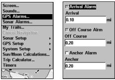
Alarms command (left); GPS alarm menu (right) with Arrival Alarm and Off Course Alarm turned on (checked).
